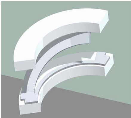
Figure 7: Final Design of Spring (1/3 rd shown)
